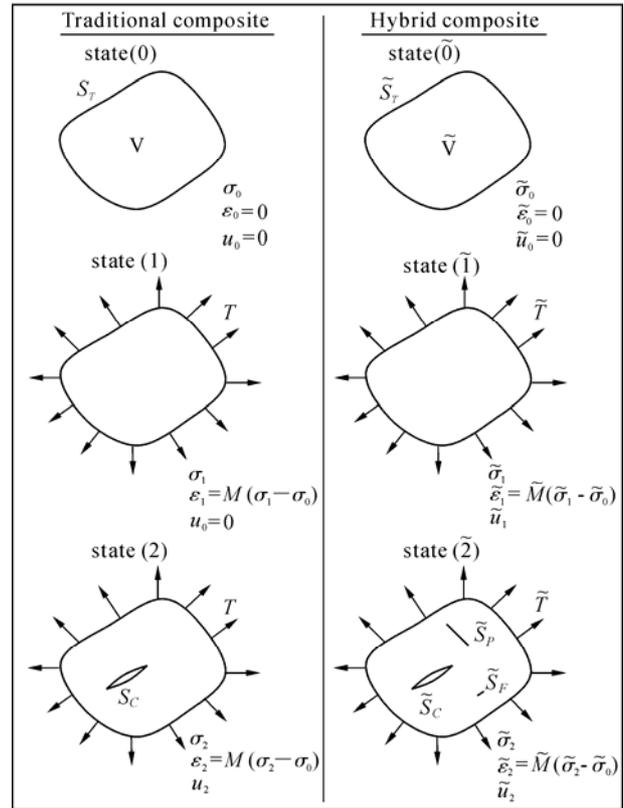
Fig.9 The three states of the body for traditional and hybrid composites. In state (2), the body has undergone some internal cracking resulting in crack surface  $S_C$ , and new values of stress distribution  $\sigma_2$ , displacements  $u_2$ , and strains  $\varepsilon_2$ .
