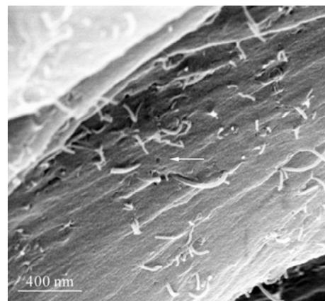
Fig.5 SEM image of fracture surface of glass fiber composite containing carbon nanotubes showing fractured and pulled-out CNTs; the arrow points to a hole from which a nanotube was pulled out
