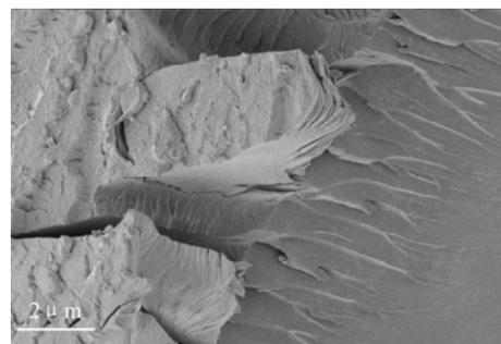
Fig.3 Fracture surface of the CNT-modified epoxy matrix
